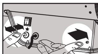
3. Press the gas button and, keeping it pressed, repeatedly press the electric piezo lighter.
