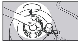
•Sluk for gasflasken.
